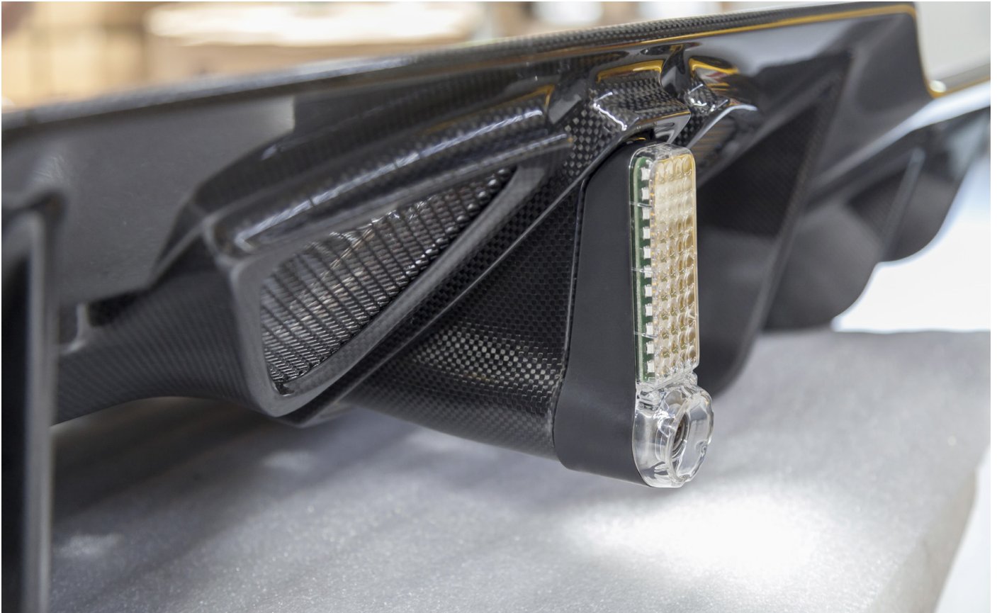
Kameraeinheit in den Diffusor einführen. / Insert the cam unit into the diffusor.
